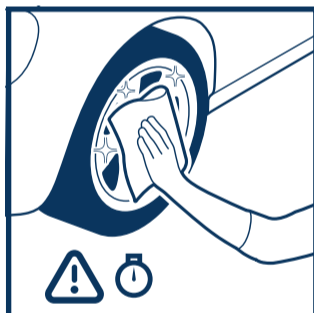
Wipe off immediately after application (ask your supplier for advice). Split complex-shaped rims in sections.
